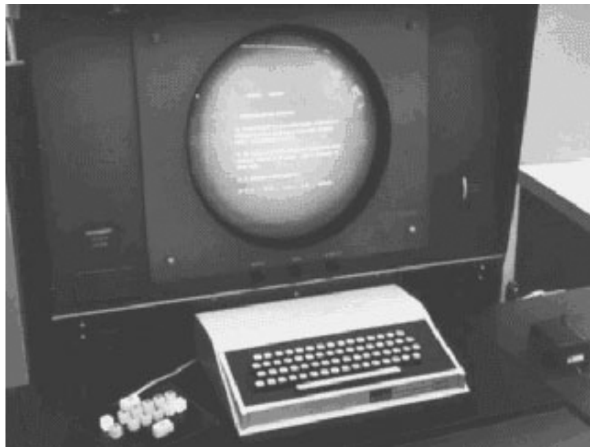
The oN-Line System display, keyboard and mouse
